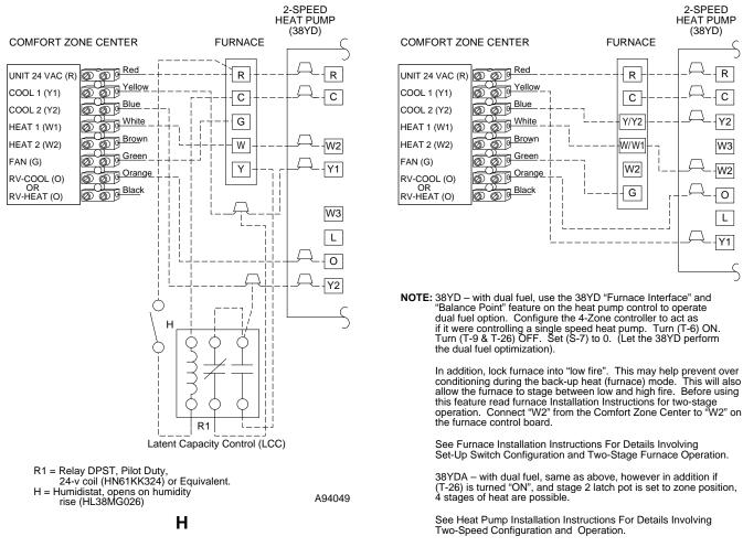
Fig. 22—Typical Wiring Diagrams (Furnace with Heat Pump) Continued
